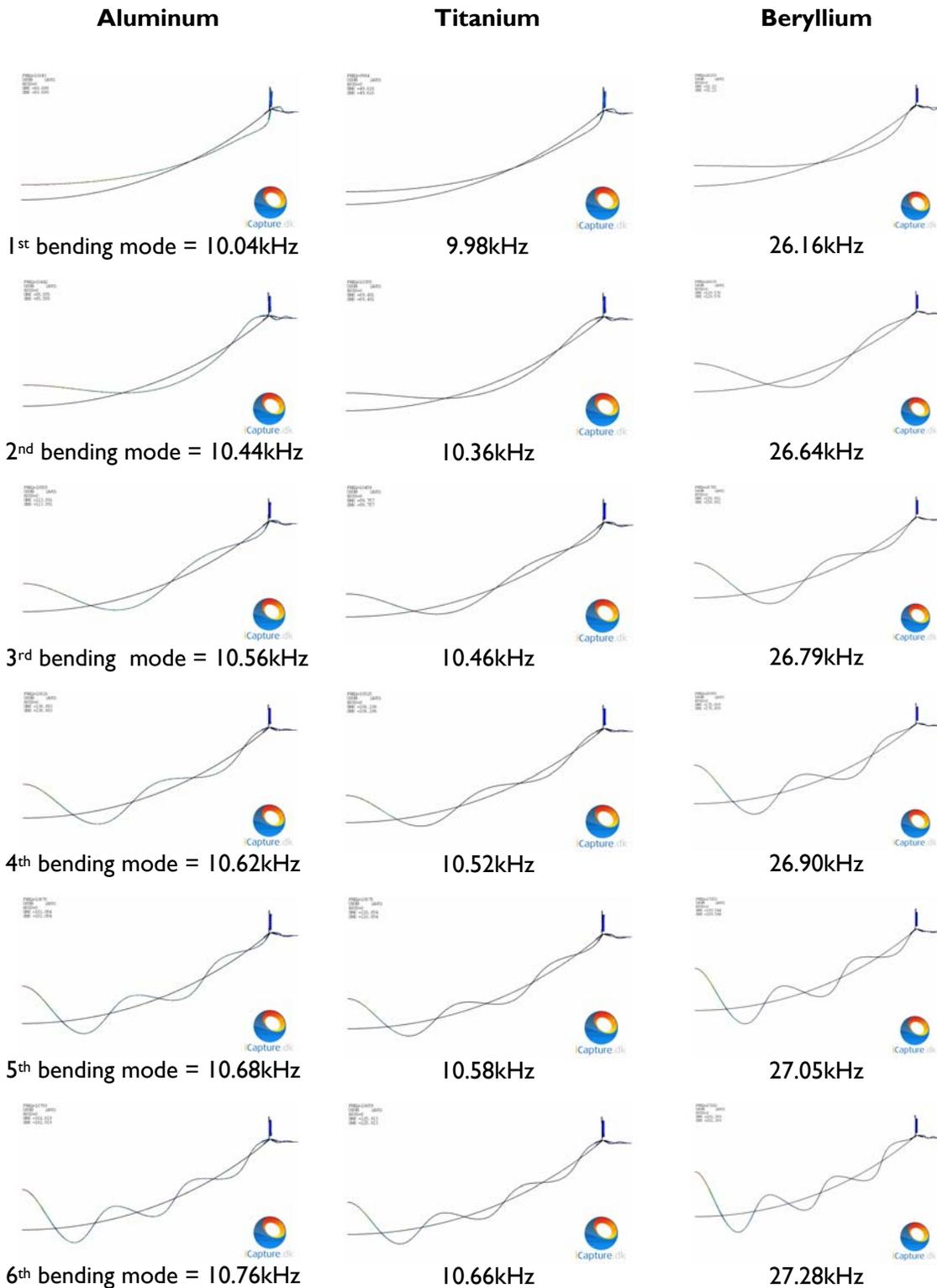
Figure 4. Bending Modes of 4” Compression Domes in Vacuo.
