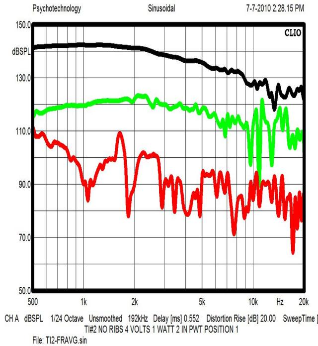
**Figure 9. Response and Distortion - Titanium Nonribbed Diaphragm.**
