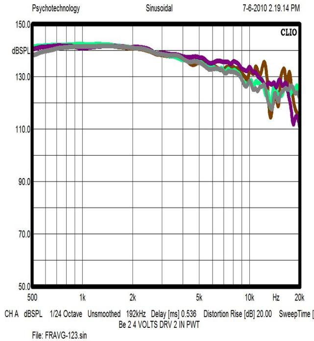
Figure 15. Response - All Four Diaphragms on a 100dB Scale. (Beryllium-purple; Aluminum-grey; Nonribbed Titanium-lime; Ribbed Titanium-brown)
