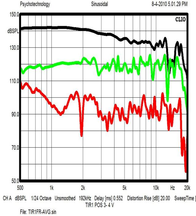
**Figure 10. Response and Distortion - Ribbed Titanium Diaphragm.**
