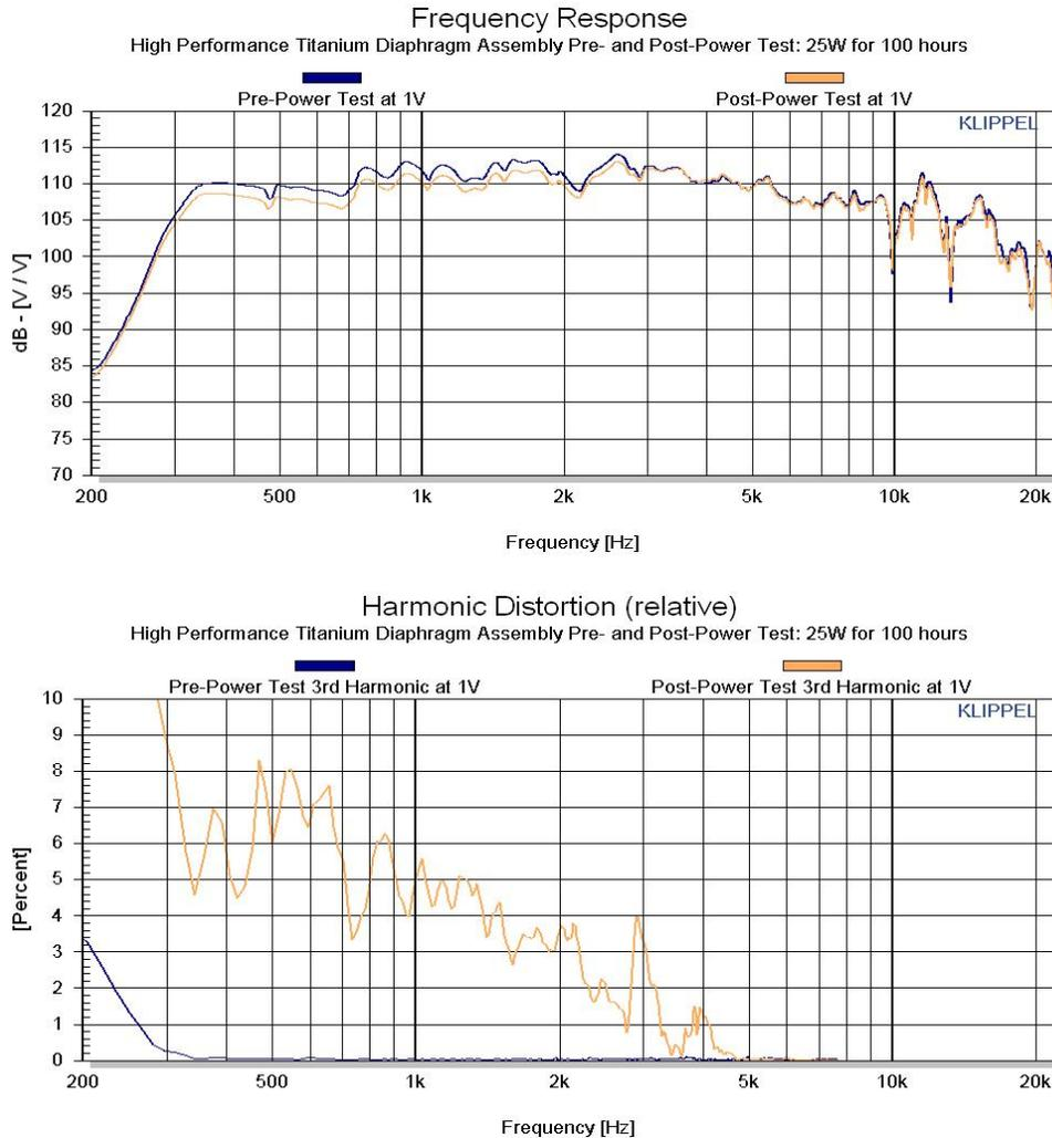
**Figure 3. Accelerated Life Test Data; Titanium Diaphragm Assembly.**
