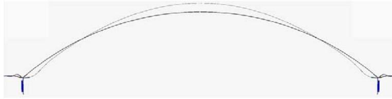
Figure I. 2D Mode Shape at 1<sup>st</sup> Bending Frequency of a Dome Diaphragm.
