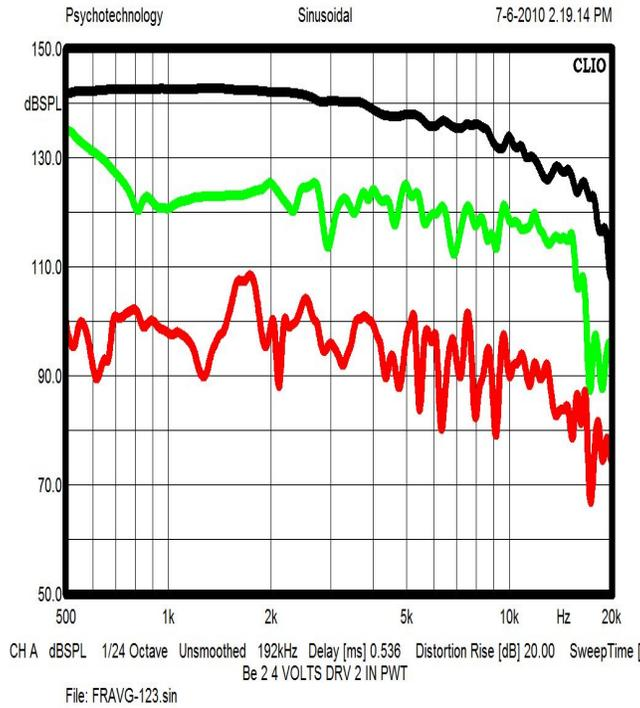
**Figure 11. Response and Distortion - Beryllium Diaphragm.**
