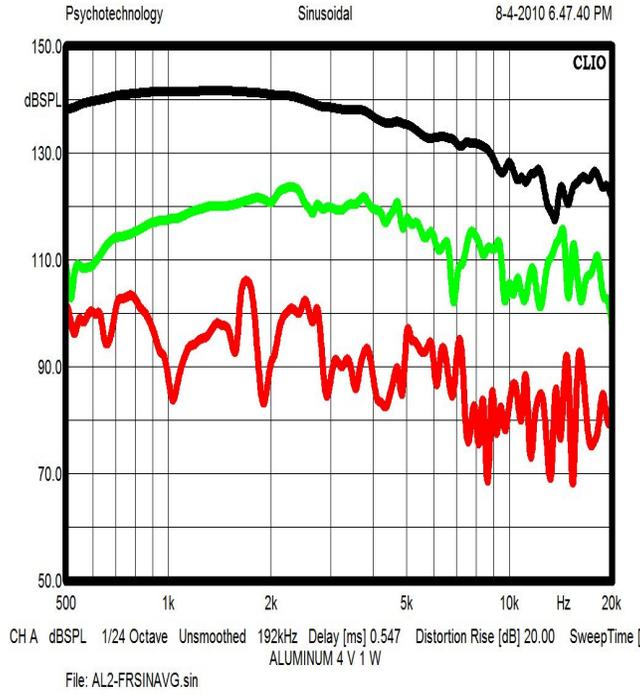
**Figure 8. Response and Distortion - Aluminum Diaphragm.**
