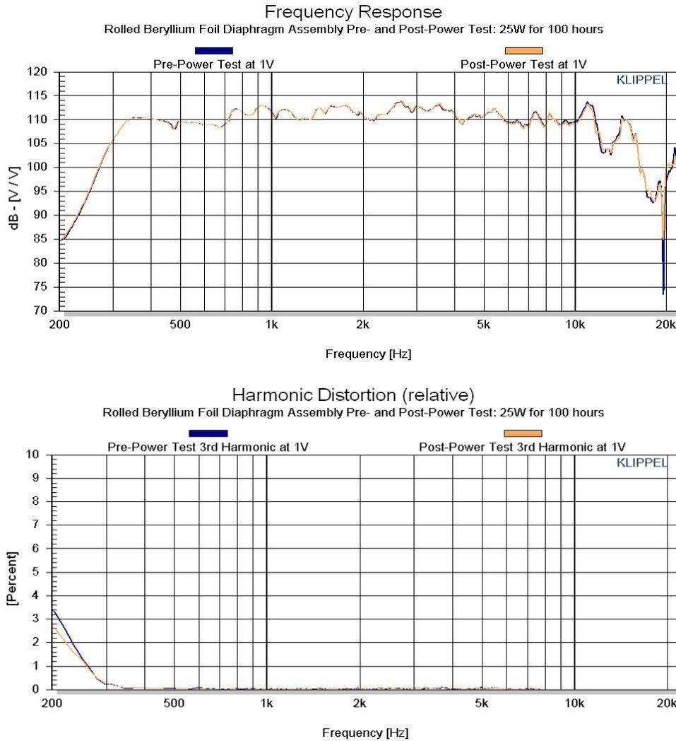
**Figure 2. Accelerated Life Test Data; Rolled Beryllium Foil Diaphragm Assembly.** 500Hz – 5,000Hz Pink Noise, 6dB CF, 12dB/octave slope. Note very small changes in frequency response and minimal increase in distortion after 100 hour test.
